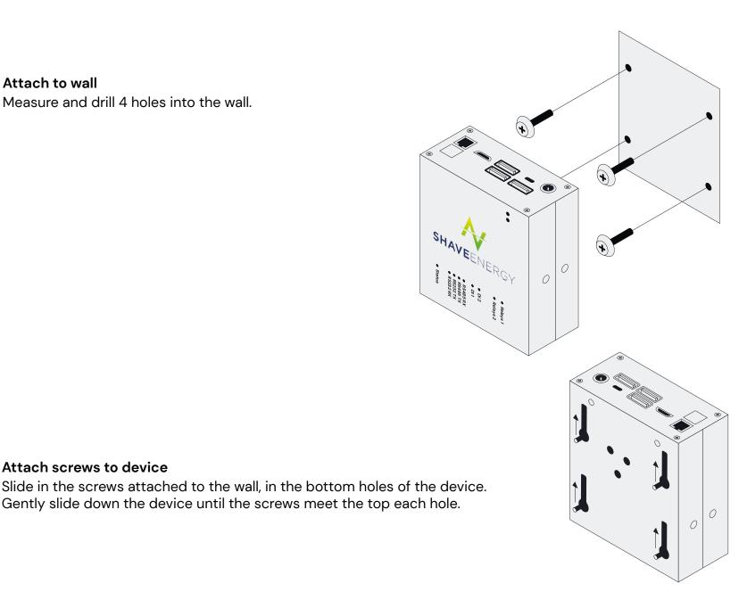
2 Attach screws to device
